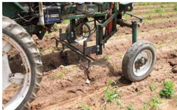
Figure 8. Side-knives removing weeds
