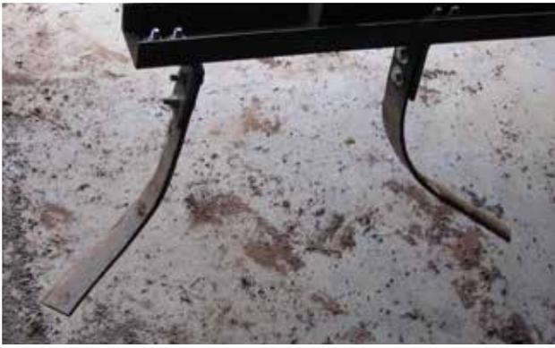
**Figure 3.** Side-knives for weed control on sides of raised beds
