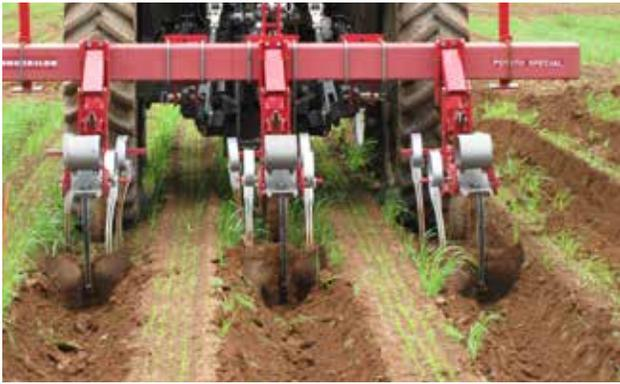
**Figure 4.** S-tines with shovels for weed control between the raised beds
