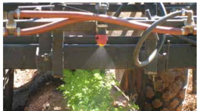
Figure 2. Banding herbicide spray on carrots
